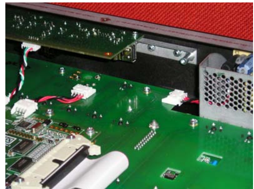
Remove the cover plate to expose the USB connector
